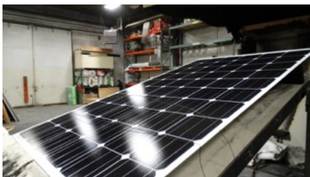
Figure 1. Photovoltaic module setup prior to burning brand test.
